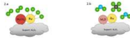
Figure 2. Methanation phase: (a) adsorption of H 2 on Ru and (b) reaction of M x CO 3 with H 2 to produce CH 4 , H 2 O and M x O.
