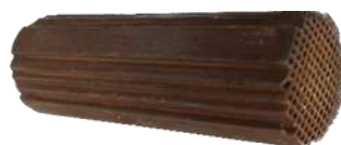
Figure 1 Structured catalyst: Sn/Pt/MgO/Al 2 O 3 /SiC
