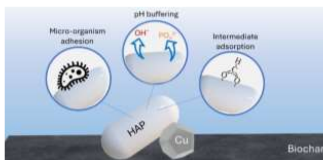
Figure 1. Schematic diagram of the role of hydroxyapatite on CO 2 electroreduction
